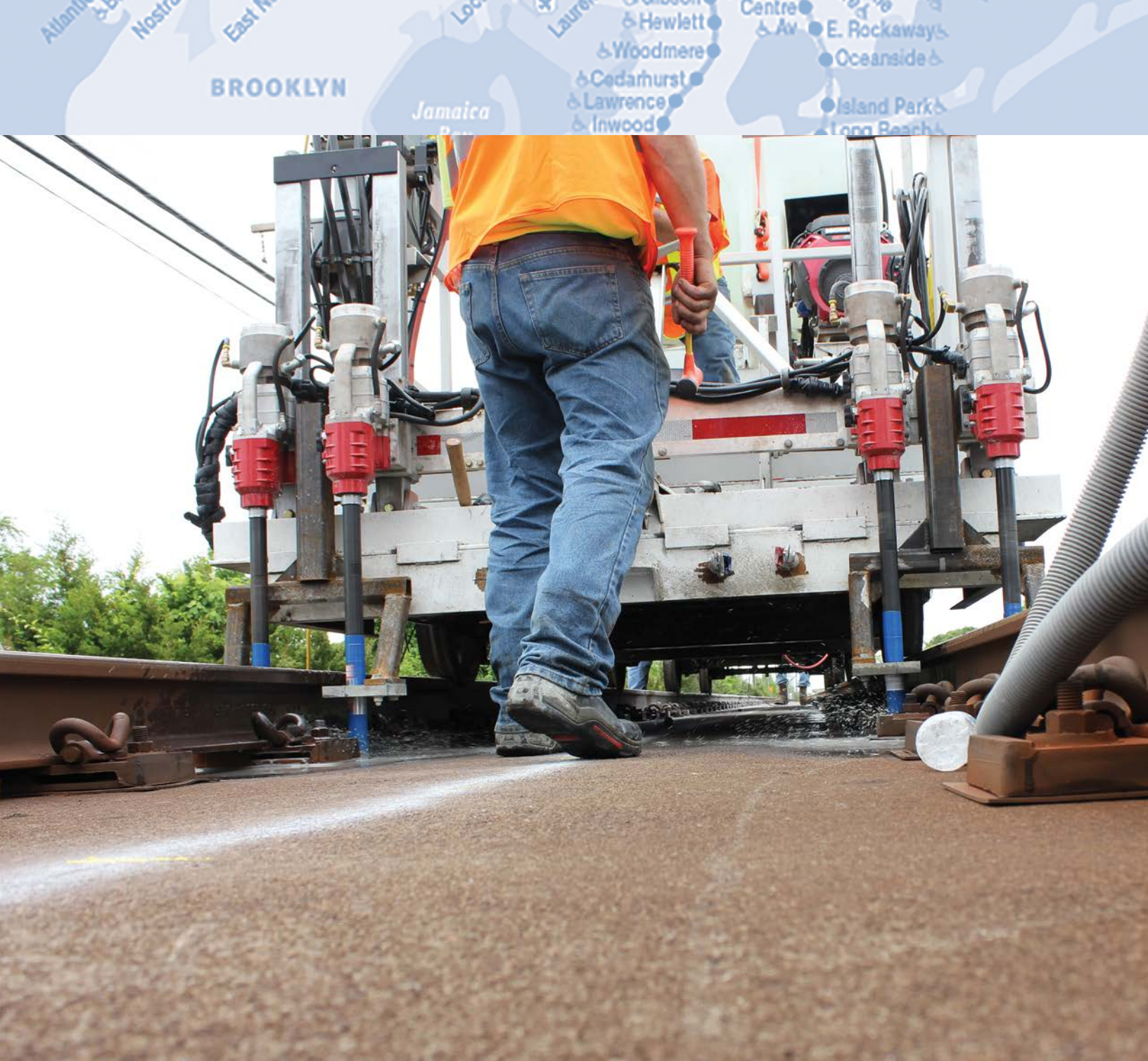
The LIRR Railcar allowed the drilling team to create four core holes at one time.
